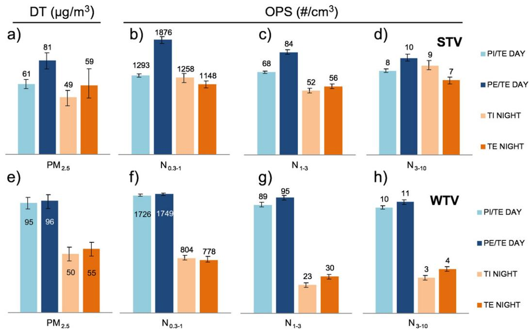
**Fig. 2.** DustTrak (DT, PM<sub>2.5</sub>) and OPS (N<sub>0.3-1</sub>, N<sub>1-3</sub>, N<sub>3-10</sub>) data for DAY (Operating hours (05:00–24:00)) and NIGHT (Non-operating hours, no platform ventilation) periods during stronger and weaker ventilation (SV/WV). PI = Platform Impulsion; PE = Platform Extraction; TI = Tunnel Impulsion; TE = Tunnel Extraction. STV: Stronger Tunnel Ventilation (summer: 49 Hz); WTV: Weaker Tunnel Ventilation (colder season: 24 Hz).
